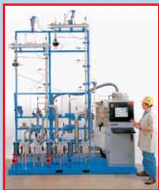
Complete turnkey 2-stage pressurizable Continuous Fractional Distillation System with 1 1/2" and 2 1/2" columns, thermosiphon reboilers, transfer pumps and receivers, explosion-proof PC-based control system.
